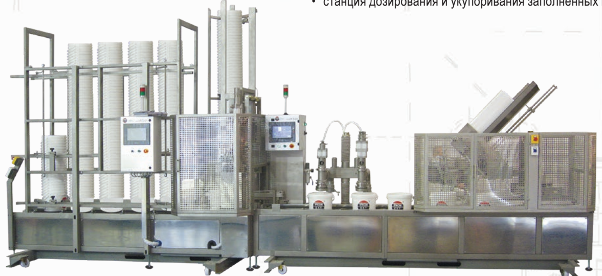
Overall dimensions LR.5 lines with buckets feeder (LxBxH), mm: 6600x1500x3500.
